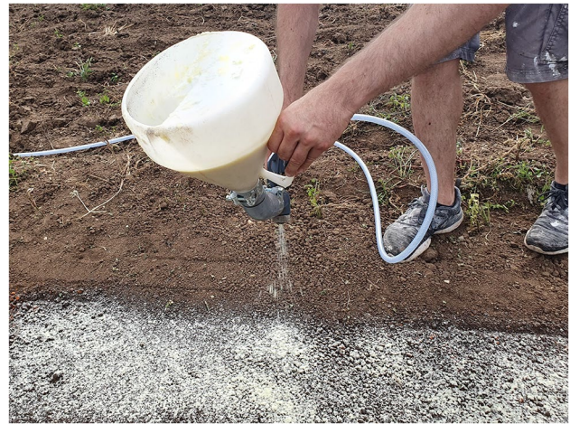
Fig. 1 Application of the mulch material with an air brush for the field trial
