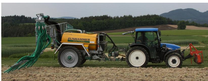
Figure 1: Slurry barrel with computer controlled drag hoses in Ascha
