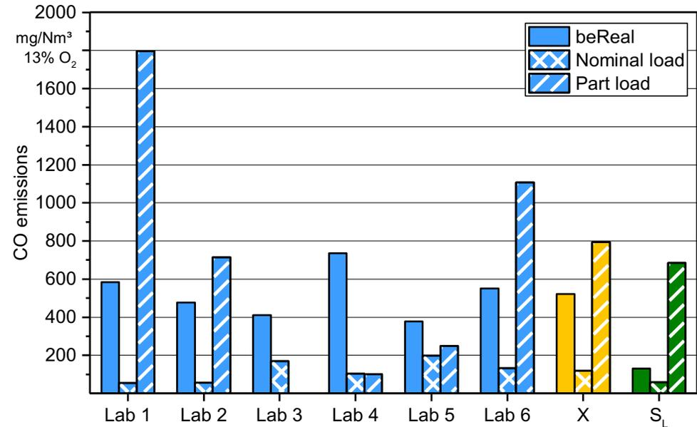
Results from round robin measurements with uniform test fuel
