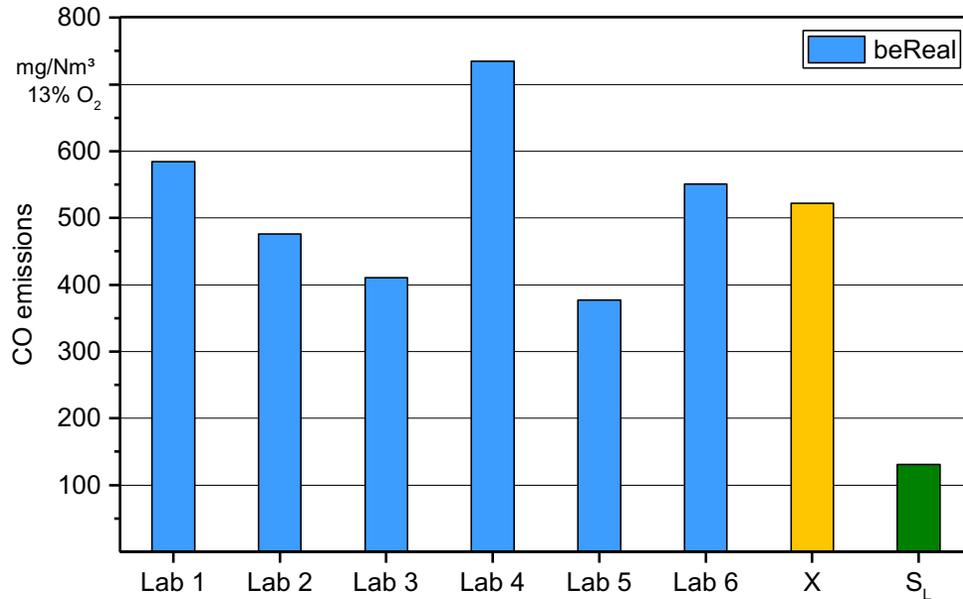
Results from round robin measurements for beReal method with test fuel for CO emissions for:
