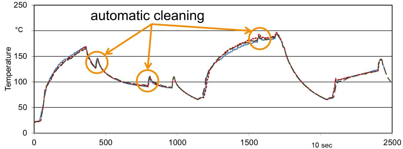
Pellet stove B 1 flue gas temp. — Pellet stove B 3 flue gas temp.
