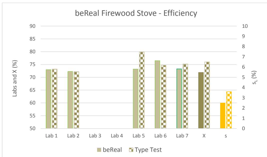
Figure 39 – Comparison of the beReal method and type testing for efficiency using test fuel.
