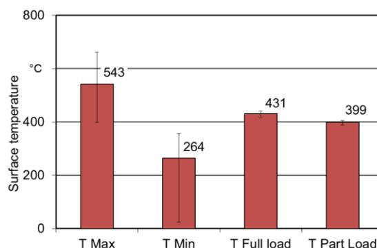
**Figure 17:** Minimum, maximum and average temperatures at full load and partial load measured at the surface of the catalytic foam ceramic element
