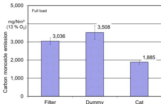
**Figure 11:** Comparison of the CO emissions for the foam ceramic filter, the catalyst and the dummy at full load operation
