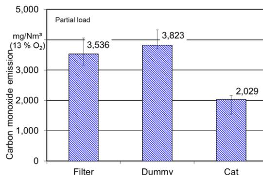
**Figure 12:** Comparison of the CO emissions for the foam ceramic filter, the catalyst and the dummy at partial load operation
