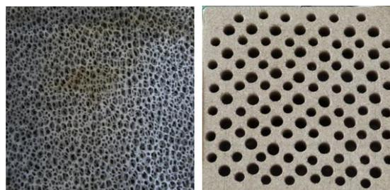
**Figure 2:** Catalytic foam ceramic (left), “Dummy”-element for achieving equal flow conditions (right)
