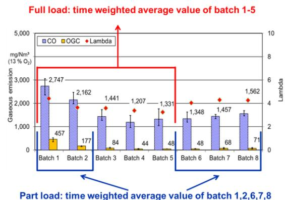
**Figure 5:** Evaluation scheme of the “close to real life” testing cycle
