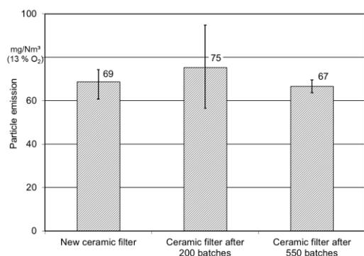
**Figure 10:** Particle emissions using three differently aged foam ceramic filters for partial load operation
