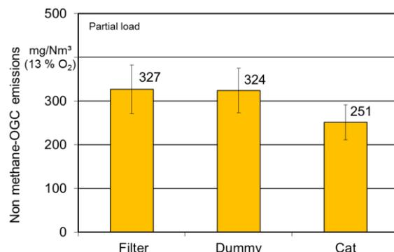
**Figure 14:** Comparison of the non-methane OGC emissions for the foam ceramic filter, the catalyst and the dummy at partial load operation
