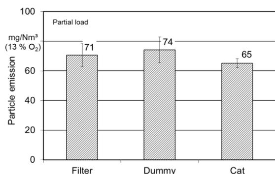
**Figure 16:** Comparison of the particle emissions for the foam ceramic filter, the catalyst and the dummy at partial load
