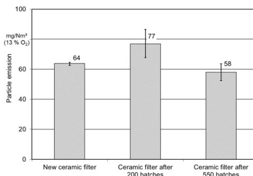
**Figure 9:** Particle emissions using three differently aged foam ceramic filters for full load operation
