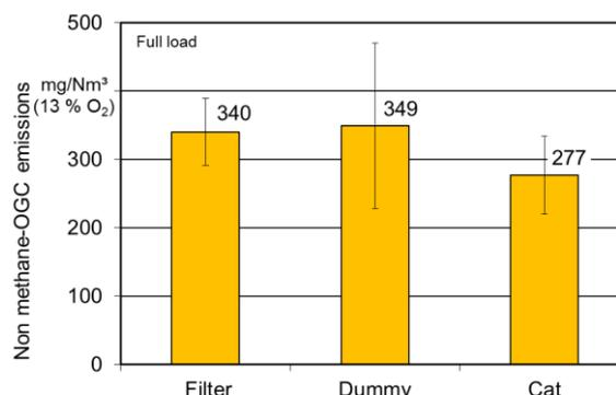
**Figure 13:** Comparison of the non-methane OGC emissions for the foam ceramic filter, the catalyst and the dummy at full load
