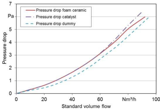
**Figure 3:** Validation of similar pressure drop achieved with all build-in components used
