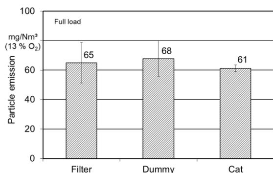
**Figure 15:** Comparison of the particle emissions for the foam ceramic filter, the catalyst and the dummy at full load operation
