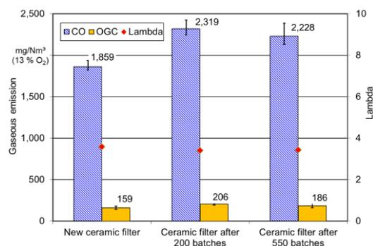
**Figure 8:** Gaseous emissions using three differently aged foam ceramic filters for partial load operation
