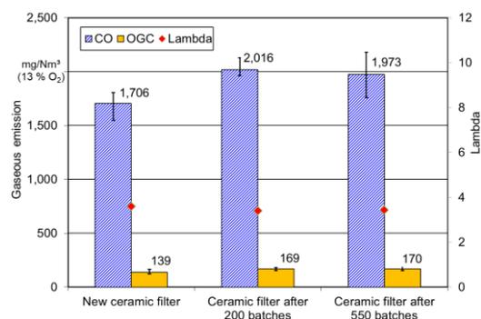
**Figure 7:** Gaseous emissions using three differently aged foam ceramic filters for full load operation
