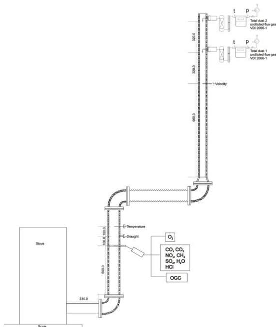
**Figure 4:** Test stand with flue gas tract for flue gas emission measurements
