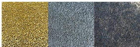
**Figure 1:** Foam ceramic filters applied: unused element (left), 200 batches (middle), 550 batches (right)
