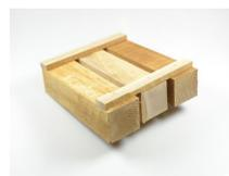
**Figure 3:** Beech wood logs without bark in test fuel shape
