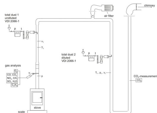
**Figure 2:** Test stand with flue gas tract and dilution tunnel for flue gas emission measurements
