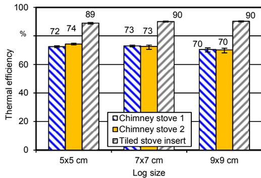
**Figure 10:** Influence of log size on thermal efficiency using beech wood in the shape of the test fuel with varying edge lengths in three stoves but applying uniform fuel masses
