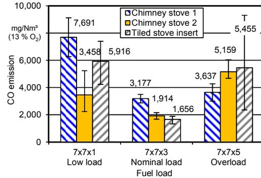
**Figure 11:** Influence of fuel amount loaded on CO emission using beech wood in the shape of the test fuel with an edge length of 7 x 7 cm in three stoves
