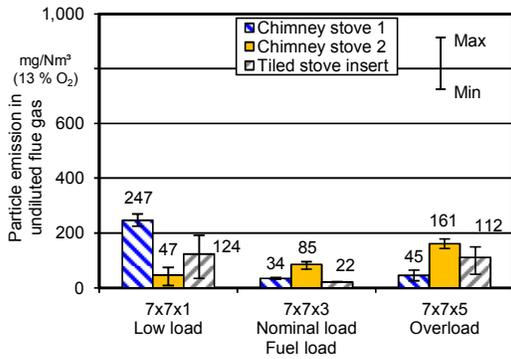
**Figure 13:** Influence of fuel amount loaded on particle emission in the undiluted flue gas using beech wood in the shape of the test fuel with an edge length of 7 x 7 cm in three stoves
