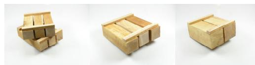
**Figure 4:** Beech wood with different log sizes in cuboid "test-fuel" shape at a constant mass
