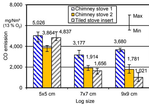
**Figure 6:** Influence of log size on CO emission using beech wood in the shape of the test fuel with varying edge lengths in three stoves but applying uniform fuel masses
