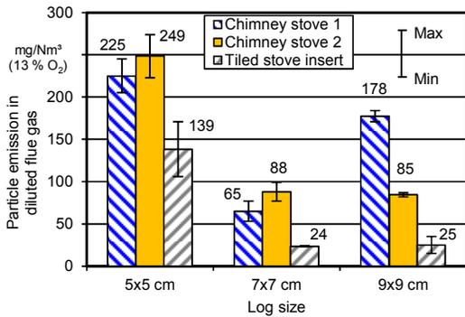
**Figure 9:** Influence of log size on particle emission in the diluted flue gas using beech wood in the shape of the test fuel with varying edge lengths but applying uniform fuel masses
