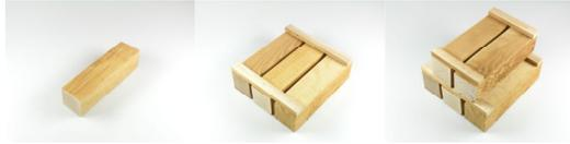
**Figure 5:** Beech wood without bark using different fuel masses per batch.
