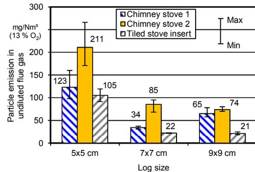
**Figure 8:** Influence of log size on particle emission in the undiluted flue gas using beech wood in the shape of the test fuel with varying edge lengths but applying uniform fuel masses
