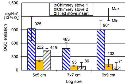
**Figure 7:** Influence of log size on OGC emission using beech wood in the shape of the test fuel with varying edge lengths in three stoves but applying uniform fuel masses
