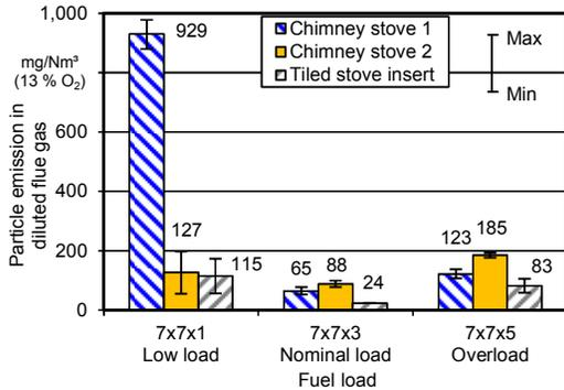
**Figure 14:** Influence of fuel amount loaded on particle emission in the diluted flue gas using beech wood in the shape of the test fuel with an edge length of 7 x 7 cm in three stoves
