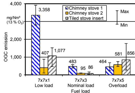
**Figure 12:** Influence of fuel amount loaded on OGC emission using beech wood in the shape of the test fuel with an edge length of 7 x 7 cm in three stoves
