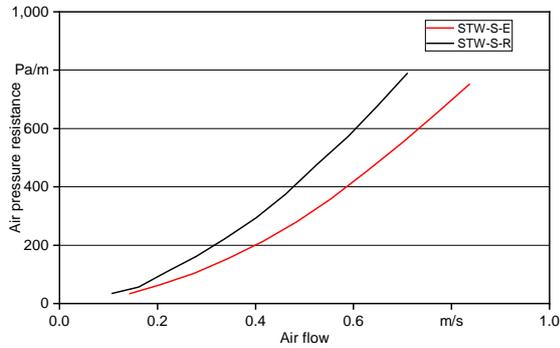
**Figure 10:** Example for differences in air pressure resistance of Effits and conventional wood chips related to the air flow rate
