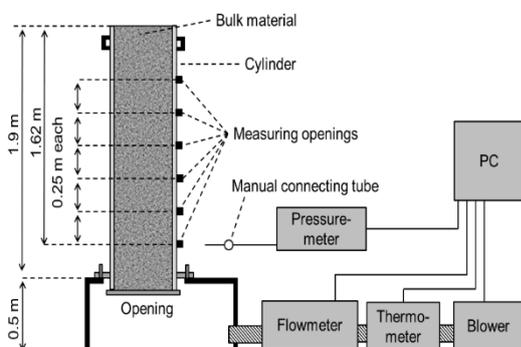
**Figure 4:** Schematic design of the air pressure resistance test stand used at the TFZ
