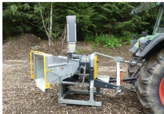
**Figure 1:** The Effiter 20.30 duplex-spiral chipper powered by a conventional farm machine.
