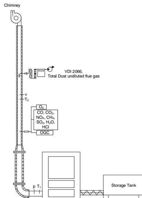
**Figure 5:** Schematic drawing of the combustion test stand used at the TFZ (position of measurement points: T = temperature, p = pressure, v = velocity)
