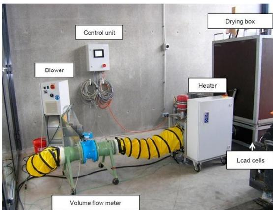
**Figure 3:** Experimental setup of the batch drying
