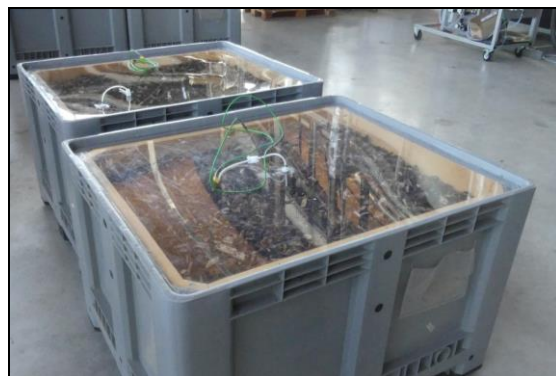
Figure 1: Wood chip storage container (anaerobic variant) with insulation and Plexiglas® sealing
