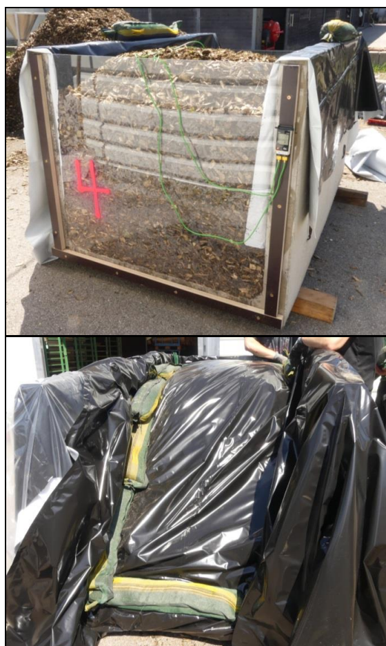
Figure 2: Small-scale silos for the storage of wood chips (top: silo during build-up; bottom: covering of a silo with wrapping foil and silage foil)
