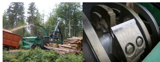
Figure 1: Chipping with the self-propelled Albach Diamant 2000 (left) was carried out with new and sharp knives (right)
