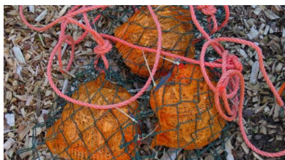
Figure 4: Balance bags for the measurement of dry matter losses and changes in moisture content
