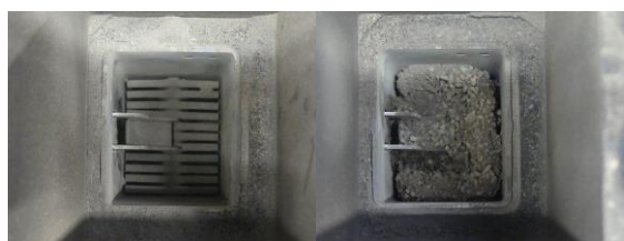
Figure 7: Combusting chamber; left: clean and empty; right: after shutdown combusting contaminated pellets filled with ash and slag
