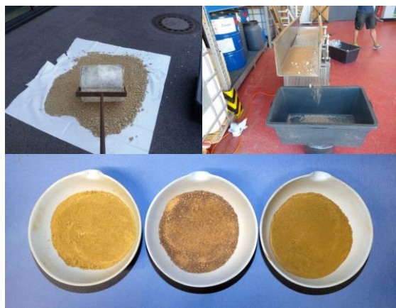
Figure 2: Preparation of soil; left top: crushing with a concrete drum; right top: screening at 2 mm with a self-constructed vibration screen; bottom, from left to right: soil A, B and C
