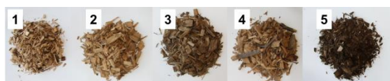
Figure 2: Five types of wood chips used for testing (Energy roundwood chips of Norway spruce (1) and European beech (2), Forest residue chips of conifer trees (3) and deciduous trees (4), Short rotation coppice chips of European poplar (5))
