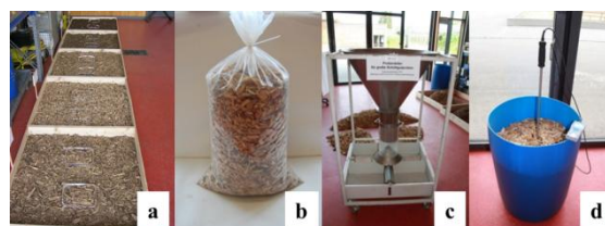
Figure 4: Measuring procedure: (a) wooden boxes for wood chip drying, (b) air-tight plastic bags, (c) sample preparation: homogenization and mass reduction, (d) barrel used for measurements with lances
