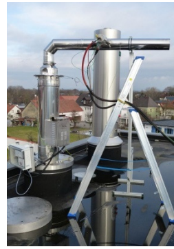
Figure 3: Scheme of field measurement setup (left) and picture of the clean gas measurement section (right)
