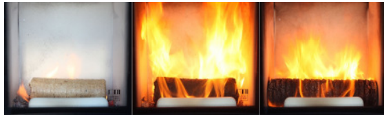
Figure 6: Wood briquettes right after recharging the stove (left) during initial combustion (middle) and finally being stuck in the firebox (right)
