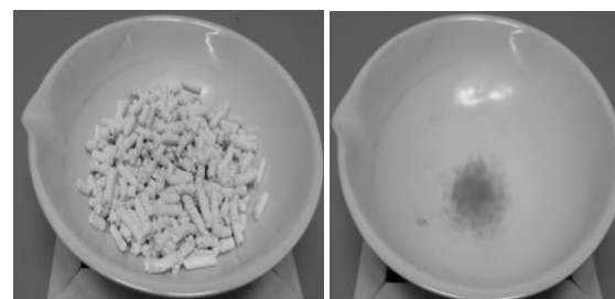
Figure 14: Wheat straw with 3.15 % kaolin after performance of the PASSA test (left) and after cleaning of the crucible by a brush (right)
