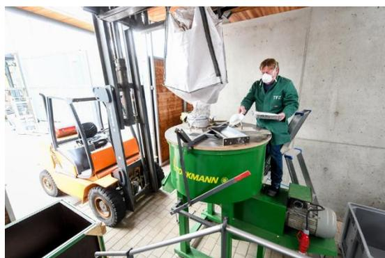
**Figure 2:** Manual additivation of milled straw fuels with kaolin in an extract mixer (© Tobias Hase, StMELF)
