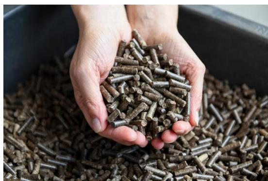
**Figure 3:** Pellets of *Carex ssp.* additivated with 1.5 w-% of kaolin (© Tobias Hase, StMELF)
