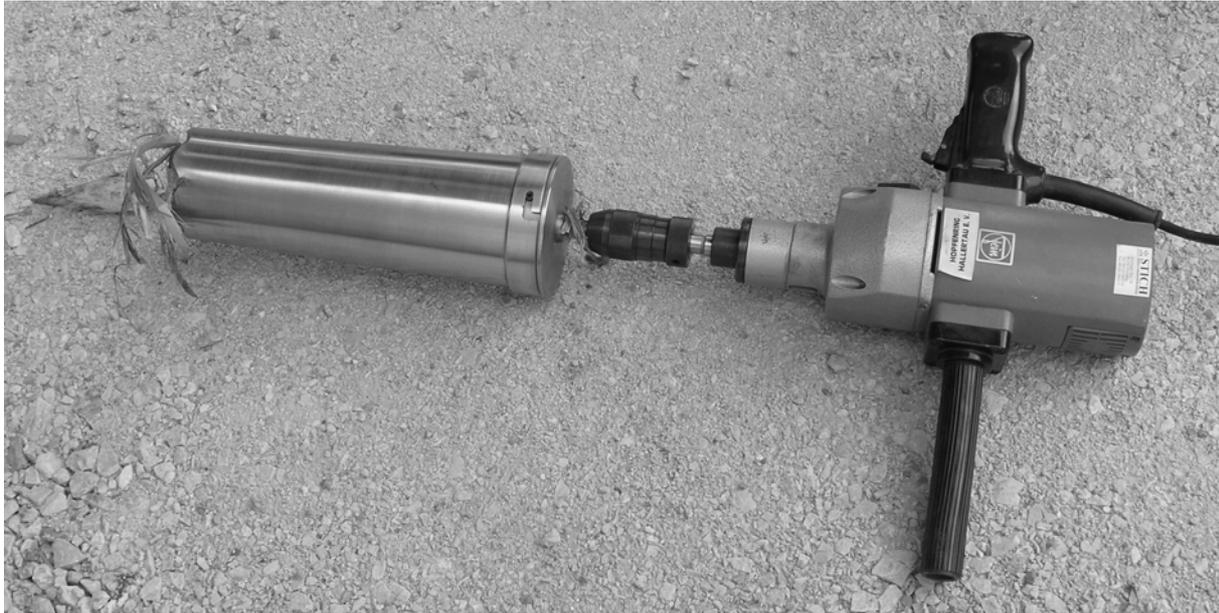
Figure 8: Core drill for maize bale samplings
