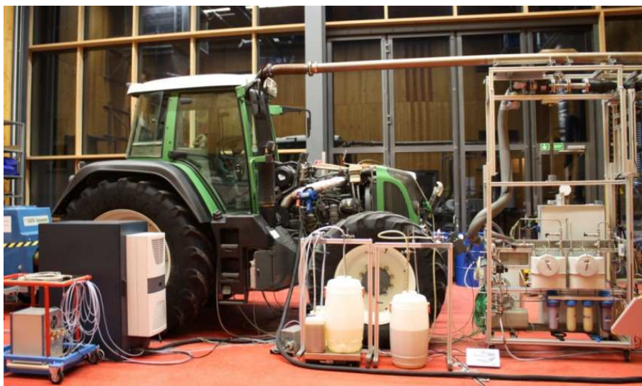
Figure 2: Vegetable oil compatible tractor at the test stand of the TFZ.
