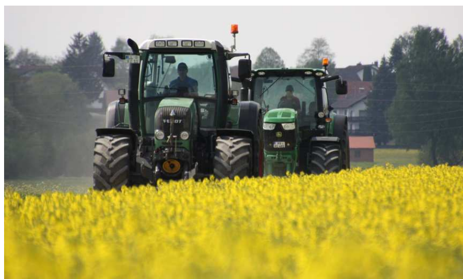
Figure 1: Vegetable oil compatible tractors - in front: Fendt 820 greentec (stage IIIA) and in back: John Deere 6210R prototype (stage IIIB).
