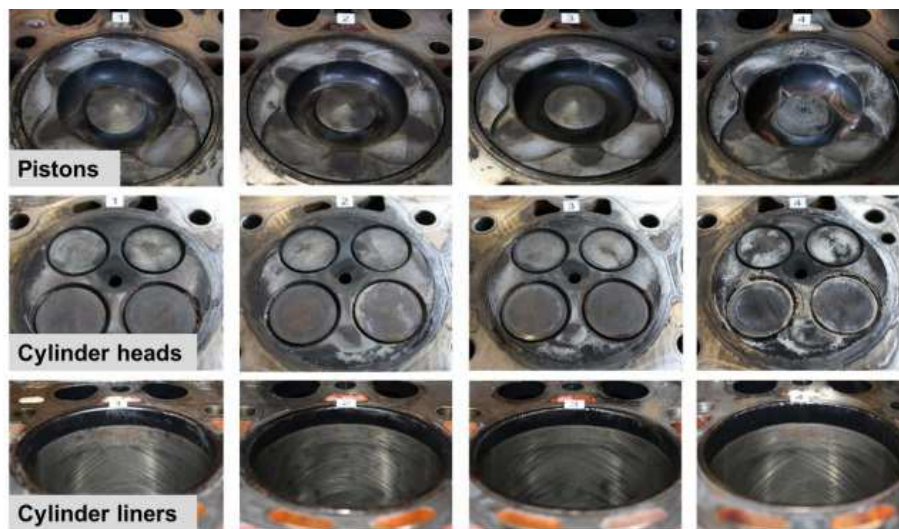
Figure 5: Pistons, cylinder head areas and cylinder liners (no. 1 to no. 4 from left to right) of tractor Fendt Farmer Vario 412 (exhaust gas stage I) at engine inspection after 5,000 h.
