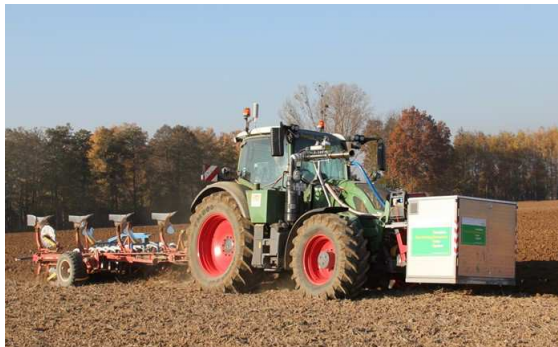
Figure 4: PEMS measurement during ploughing with a vegetable oil compatible tractor Fendt 724 SCR (Stage IV)
