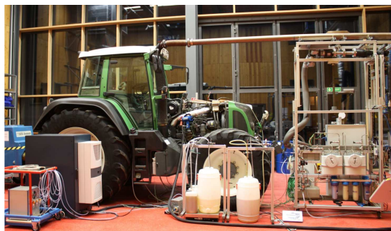
Figure 1: Plant oil compatible tractor at test stand of the Technology and Support Centre (TFZ)
