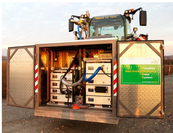
Figure 2: Set-up of portable emission measurement system PEMS Semtech Ecostar in purpose built box
