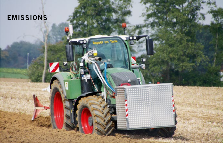
FIGURE 2 RDE measurements of a Fendt 724 S4 with PEMS during ploughing (© TFZ)
