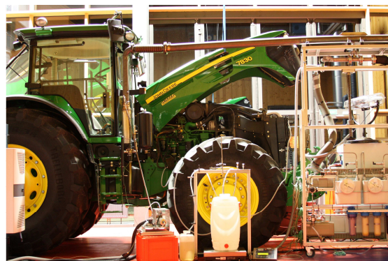
Figure 1: Plant oil compatible tractor at test stand of the Technology and Support Centre (TFZ)
