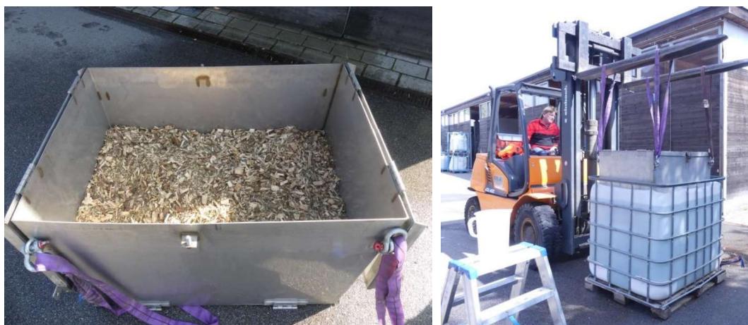
Figure 2: Washing woodchips; left: washing box with FRC; right: lifting the washing box into and out of the IBC tank;
