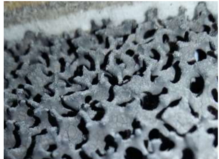
Foam ceramic after 16 days of operation
