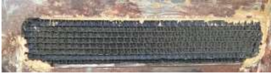
Catalyst before the test runs (view at outlet)
