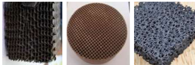
Monoliths (honeycomb or foam structure)
