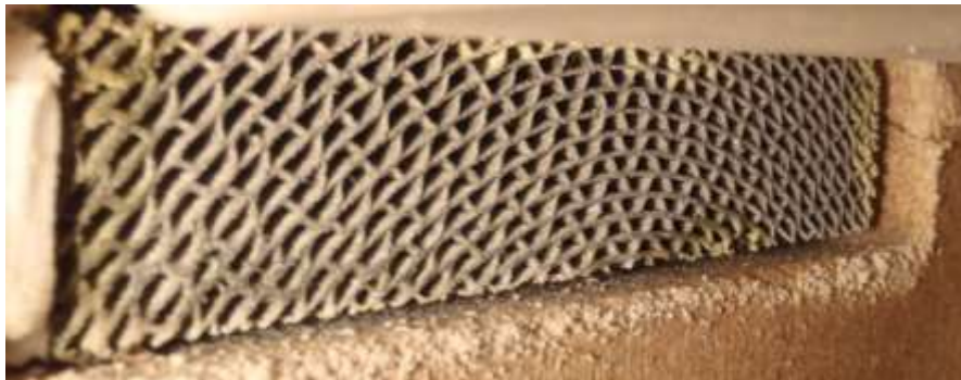
Catalyst 2 weeks of operation (view at inlet)
