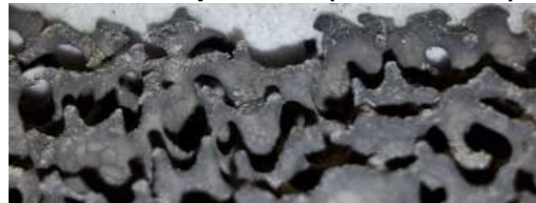
Foam ceramic after manual cleaning after 2 weeks of operation (view at inlet)
