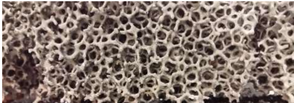
Foam ceramic after manual cleaning after 2 weeks of operation (view at inlet)
