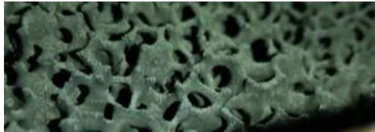
Foam ceramic after 2 weeks of operation
