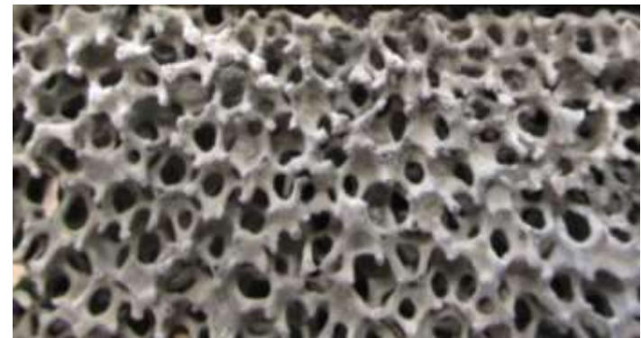
Foam ceramic after 18 days of operation
