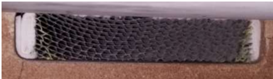
Catalyst after manual cleaning after 2 weeks of operation (view at inlet)
