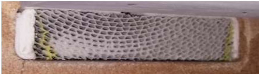
Catalyst after 2 weeks of operation (view at inlet)
