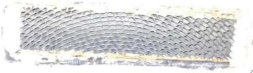
Catalyst 2 weeks of operation (view at inlet)
