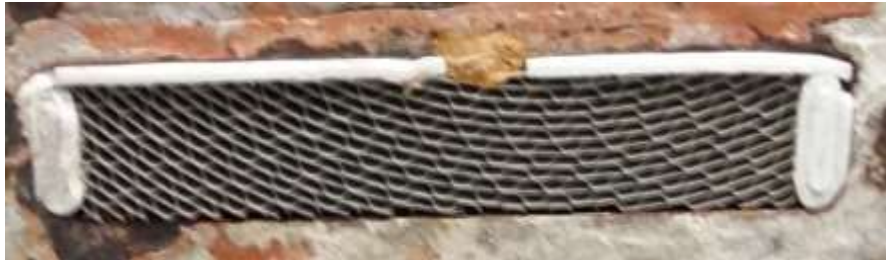
Catalyst before the test runs (view at outlet)
