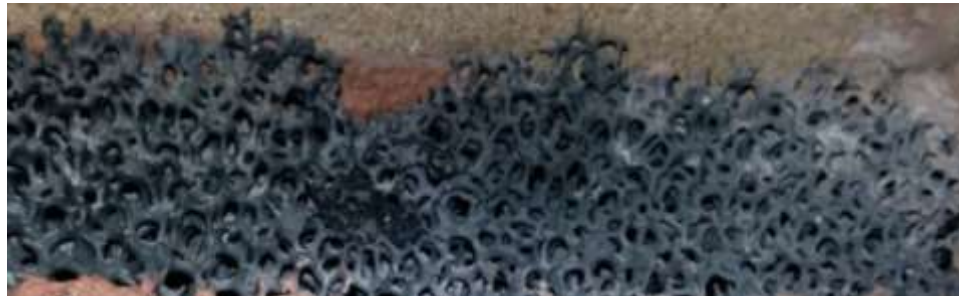
Foam ceramic after manual cleaning after 2 weeks of operation (view at inlet)
