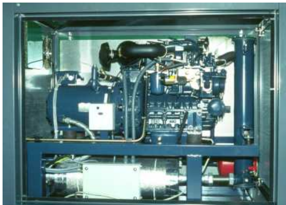
Figure 1: Vegetable oil compatible Mini-CHP plant with combustion engine (8 kW el , 16 kW th ), manufacturer: KW-Energietechnik
