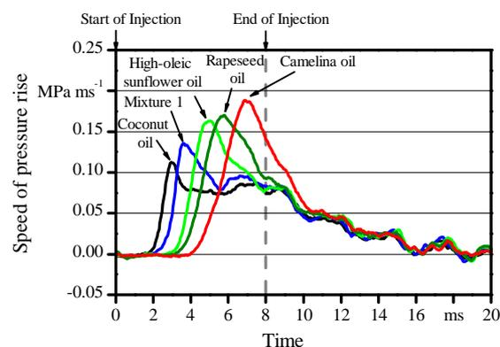
**Figure 2:** Speed of pressure rise in the combustion chamber of the FIT after injection of coconut oil, mixture 1, high-oleic sunflower oil, rapeseed oil and camelina oil
