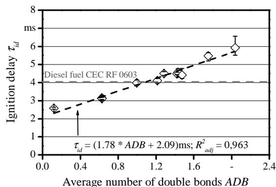
**Figure 3:** Arithmetic mean and maximum deviation of the ignition delay  $\tau_{id}$  of vegetable oils in relation to the average number of double bonds *ADB* and compared to diesel fuel
