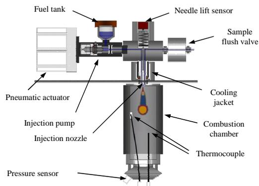
**Figure 1:** Schema of the Fuel-Ignition-Tester (FIT<sup>TM</sup>) (reference: Fueltech, modified)
