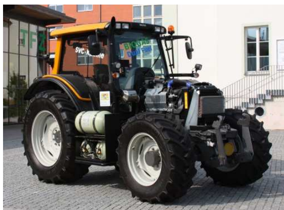
Figure 1: Dual-fuel tractor Valtra N101 HiTech for bio-methane and diesel operation
