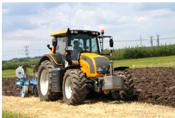
Figure 7: Prototype Valtra N101 Hi Tech dual-fuel tractor in practice field test.
